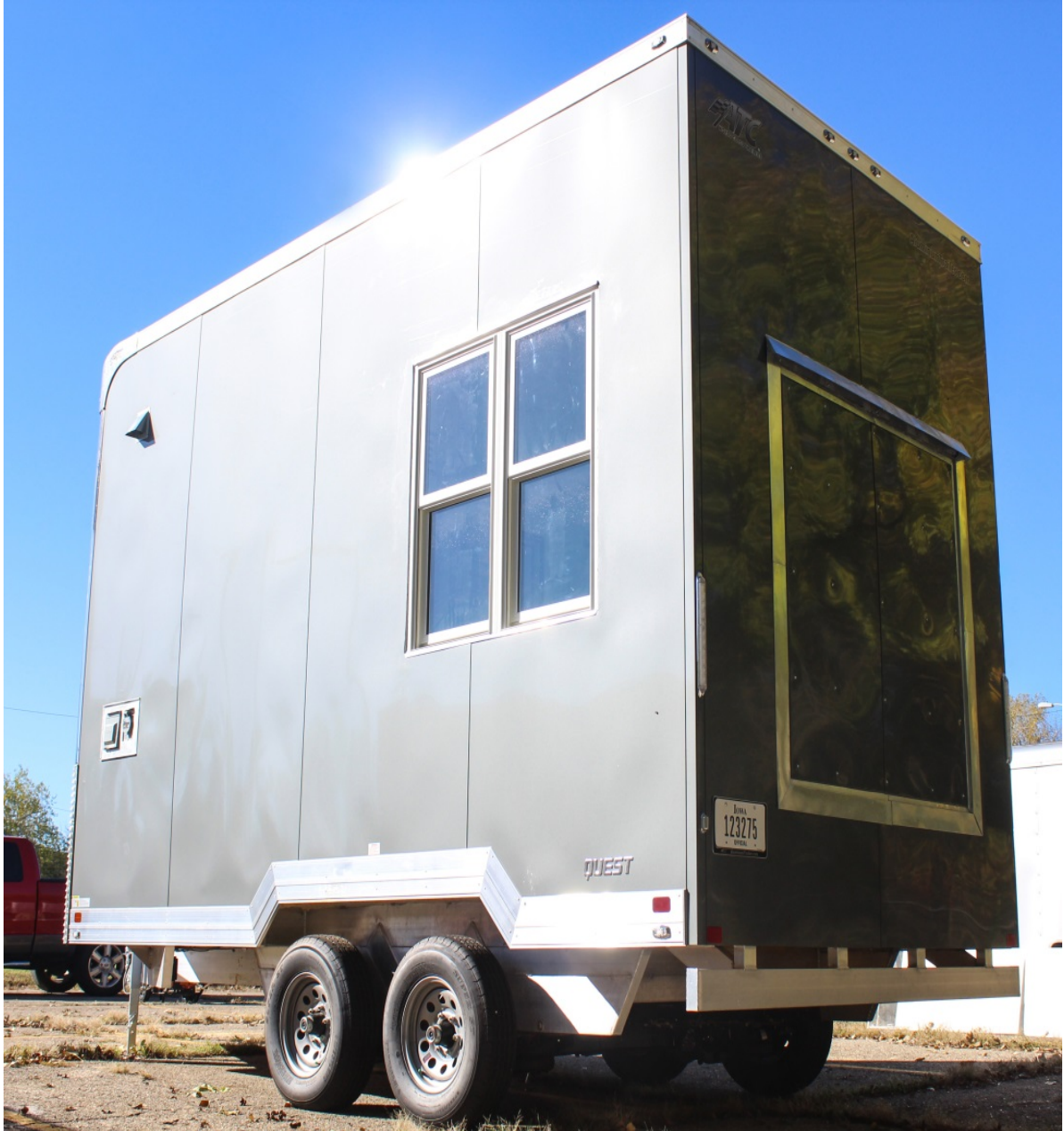
Figure 4-1 Profile of the Mobile Diagnostics Lab with removable wall panel in the rear wall.
