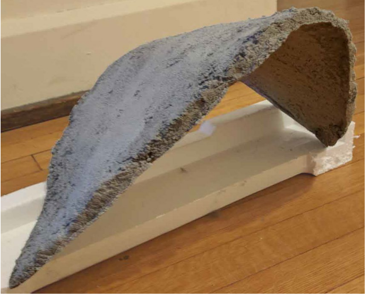
Figure 3-5 Cast concrete shells with CNC measuring 1' X 6'' X 11½'' and 1/4'' thick.
