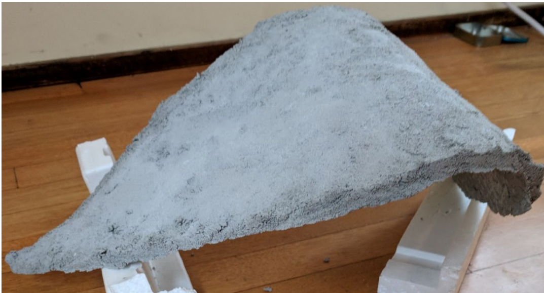
Figure 3-4 Cast concrete shell without CNC measuring 1' X 6" X 11½" and ½" thick.
