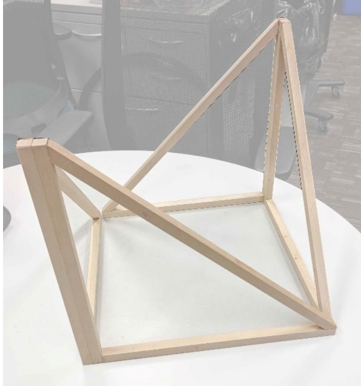
Figure 3-2 Scale wood frame model constructed with reference rhino model, grasshopper and karamba, using \frac{1}{2} "x \frac{1}{2} " basswood members.
